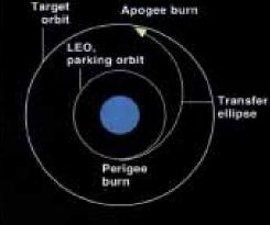
It is common procedure to pick an initial "parking" orbit, usually at LEO, then boost payloads to higher attitude. Engines are fired first (at perigee) to reach the apogee of an elliptical transfer orbit and then are fired again to put the spececraft into a circular orbit at that higher altitude.
